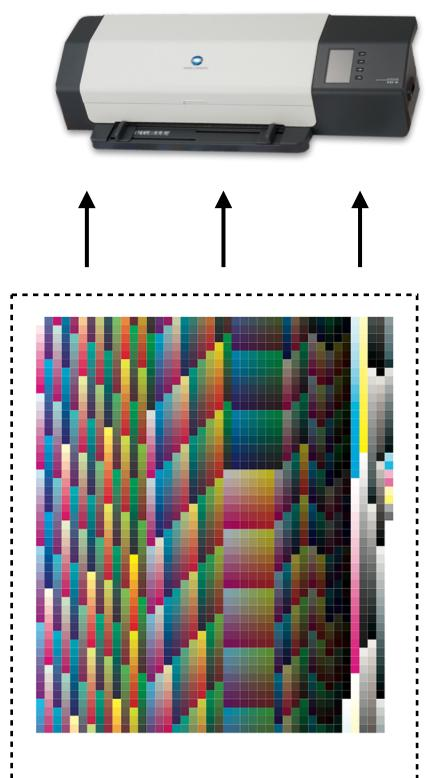
2. **FD-9** is now detecting the patches by comparing the scanned image with the reference data contained in the .xml file
